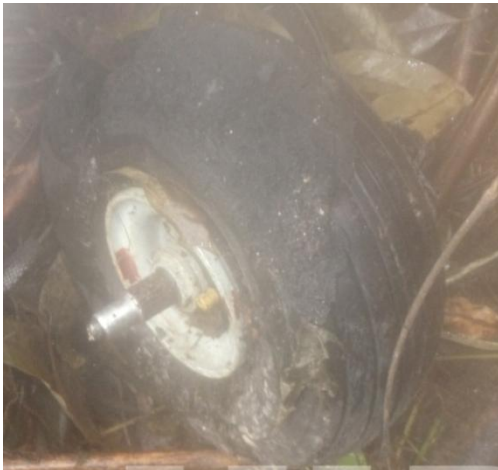
DAMAGED NOSE WHEEL
